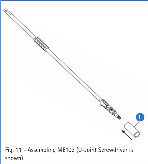
Fig. 11 - Assembling ME103 (U-Joint Screwdriver is shown)
